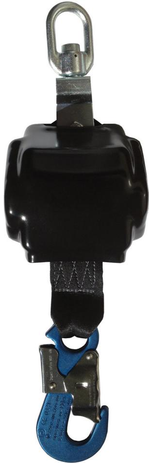
The Abtech Torq 2.4 is a small self-retracting lifeline designed to provide protection from falls from height. Anchored above the users center of gravity it gives the user a safe area of work. The retracting line pays in and out of the device allowing the user freedom of movement within the safe area.
