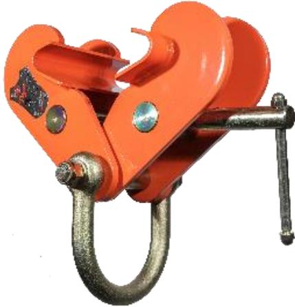
The Tiger BCF clamp has been designed as a robust anchor point suitable for pulling and lifting at angles across the beam. It allows for up to 90° side loading with no deration and 15° cross loading with no deration.
