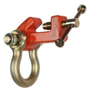
The Tiger BCB bulb bar anchor is designed for attaching to bulb profiles of bulb flat bars approved for lifting applications. These are often found in ship compartments, engine rooms and overhead bridge deck structures. The bulb bar anchor provides a semi-permanent lifting point. The large integrated shackle gives easy connection for all different types of lifting machines. This model must NOT be used for lifting beams. It is a suspension point.
