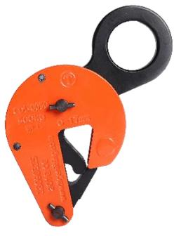
Tiger CDL drum lifting clamp has been designed to lift and transport steel drums and is lightweight and easy to use. If you are lifting empty or sealed drums, then one clamp is sufficient on its own. If you are lifting an open full drum, then two clamps should be used with a two-legged sling.
