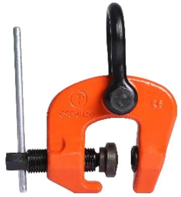
The Tiger CSC 'swivel hook' screw cam clamp is suitable for many applications. It is particularly useful for lifting and pulling sheet metal, girders, and steel constructions. It is fitted with a moveable cam on the thread spindle which provides a powerful clamping force on the object being moved.
