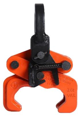
The Tiger CRT rail clamps are designed to lift lifting and pulling single rails lengthways and crossways, securely and safely. The clamps are designed to fit most types of rail section currently in use. The clamps are locked onto the rail-head via a lever operated spring mechanism. Very solid, practical design with low dead weight. For rail sizes S49, S54, S60s, UIC60.
