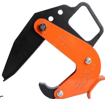
The Tiger CPL pipe lifting clamps are used in sets of three for the vertical transportation of concrete pipe sections with a diameter of up to 2m. The jaw capacity is designed for pipe thickness of 40-220mm for the 1.5t capacity set and 90-220mm for the 3.0t capacity set. Attachment and removal of the clamps from the pipe is extremely easy due to the simple and straightforward design. For concrete according to DIN4034. The working load limits shown are based on a set of three clamps.
