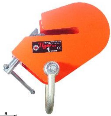
This BCA clamp serves as an anchor or lifting point when attached to an overhead steel angle section approved for lifting applications. This clamp can be used up to a maximum of 15° from the vertical.
