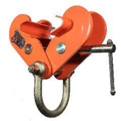
The Tiger BCF clamp has been designed as a robust anchor point suitable for pulling and lifting at angles across the beam. It allows for up to 90° side loading with no deration and 15° cross loading with no deration.
