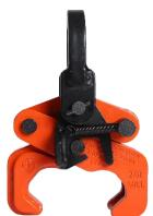
The Tiger CRT rail clamps are designed to lift lifting and pulling single rails lengthways and crossways, securely and safely. The clamps are designed to fit most types of rail section currently in use. The clamps are locked onto the rail-head via a lever operated spring mechanism. Very solid, practical design with low dead weight. For rail sizes S49, S54, S60s, UIC60.
