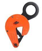
Tiger CDL drum lifting clamp has been designed to lift and transport steel drums and is lightweight and easy to use. If you are lifting empty or sealed drums, then one clamp is sufficient on its own. If you are lifting an open full drum, then two clamps should be used with a two-legged sling.
