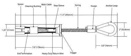
Concrete Anchors are portable, reusable devices which can be used in vertical, horizontal or overhead concrete substrate surfaces. Once a suitable hole has been drilled, the anchors can be inserted and removed as required. These anchors are available in two sizes/rating and are suitable for use for fall protection applications.
