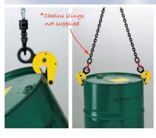
The DC500 drum clamp has been designed to lift and transport steel drums. If moving empty or sealed drums then one clamp is sufficient. Should you be lifting an open full drum, then two clamps should be used with a two leg chain sling.
