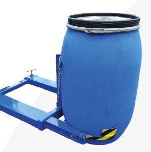
The Mauser drum grab is designed for handling 'egg-shaped' 210 litre plastic drums. Full automatic in operation, the mauser drum handler is designed to grip and secure the drum via its base during lifting. An upright support section adds additional stability to the drum.
