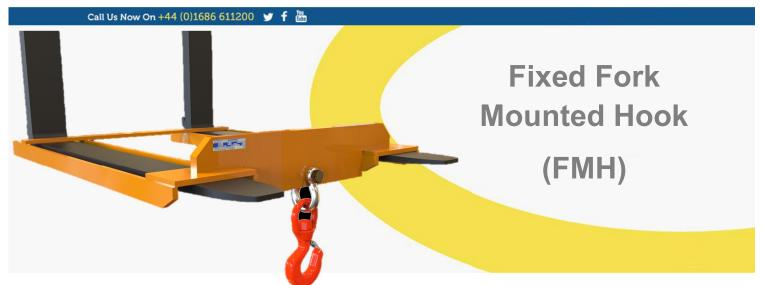
Our hugely popular Fork Mounted Hooks can be fitted to your fork truck quickly and easily; simply, lift the front of the attachment where the hook is located until the attachment is approximately at 45 degrees. The attachment can then be slid on the forks towards the carriage. When the attachment is a far back as possible lower the front down onto the forks and the retaining bar will go up behind the forks and hence the hook is ready for use.
