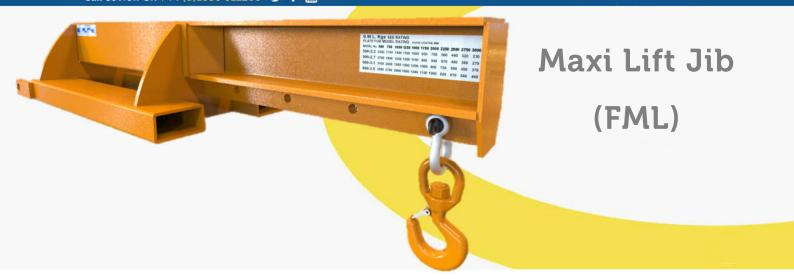
Our best selling Maxi Lift Jib is designed to offer a solution to the handling of larger, heavier loads safely. To fit, simply ensure the heel pins are removed, then drive slowly into the attachment sleeves as far as possible. Then simply re-fit the heel pin behind the forks of the truck and the jib is now ready to begin lifting.
