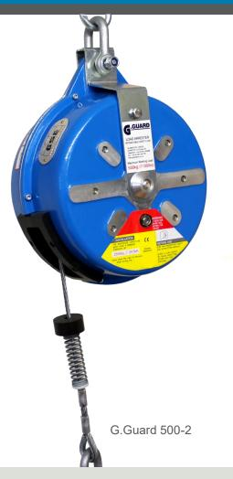
Globestock's® G.Guard series of load arrestors is a reliable system for automatically stopping the fall of an overhead load, protecting the load whilst at the same time reducing the chance of injury to anyone nearby. If the load enters into free-fall, the cable is pulled out at an accelerating rate; when the activation speed is reached, the braking system engages, bringing the load to a smooth and cushioned stop.
