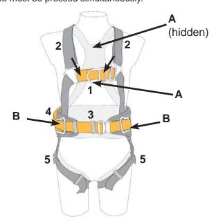
Step into harness, fasten and adjust in the order shown in the diagram.
