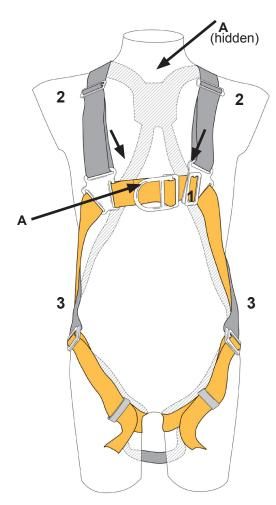
Harnesses are made from polyamide and polyester, with steel and aluminium alloy fittings.
