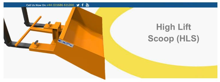
To fill the bucket and pick up a load of material, the material should be approached with the bucket at ground level. The truck is driven carefully forward, with the mast as near upright as possible until the bucket fills. The forks can then be raised and the material transported as required. To dump the material, the bucket is positioned directly over the discharge point. Once correctly positioned the operator lifts the release lever and the contents are discharged.
