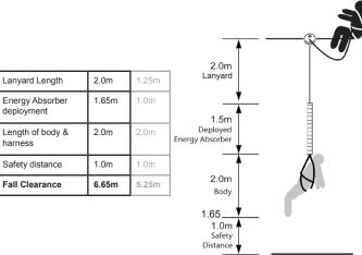
During a fall the energy absorber may deploy by up to 1.65m. Allow sufficient clearance between the anchor point and the ground or anything else below. heightec reccommend a clearance of 7.0m for 2m lanyards.
