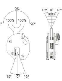
Loads weighing the maximum W.L.L may be lifted through15 degrees in the plane of the clamp
