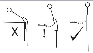
The rope protector should be inspected before each use to ensure it is in good condition, free from holes, sharp edges etc.
