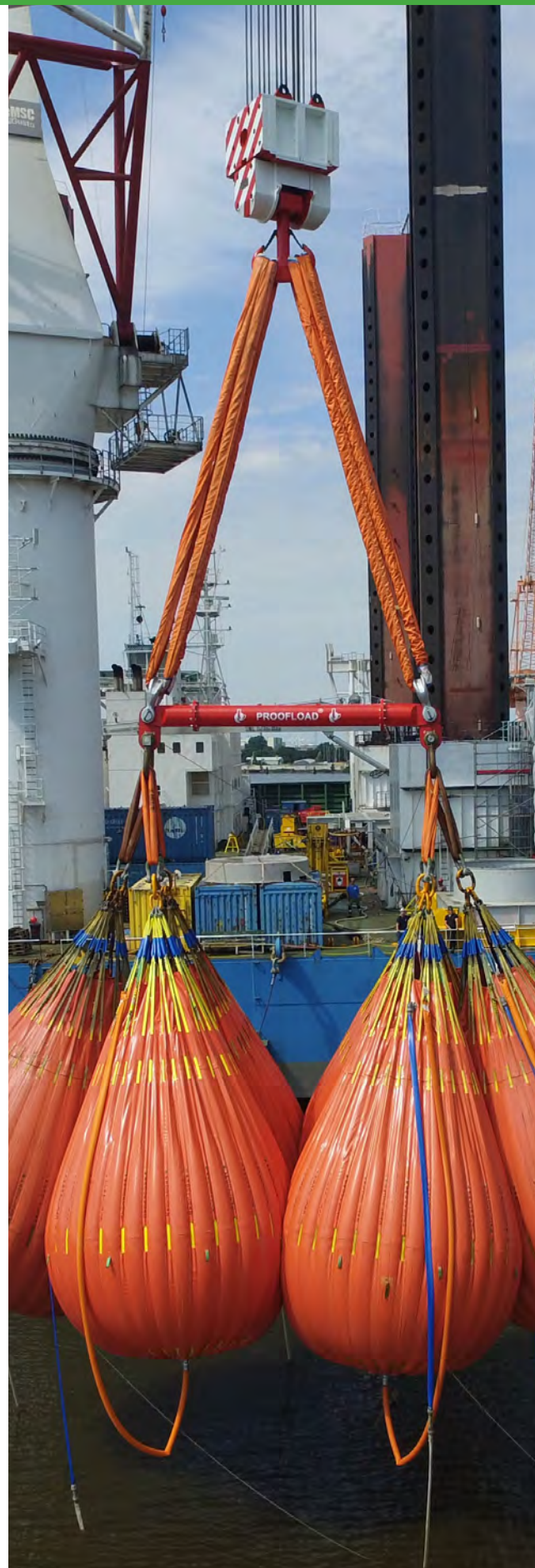
Two Miller Weblift 150T 18 metre Techlon Round Slings helping to proofload waterbags.
