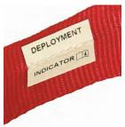
**Deployment Indicator** In the event of a shock load the deployment indicator will tear providing a visual guide to remove from service.
