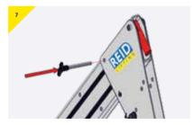
Re-insert ball-lock pin into hole ensuring the pin is fully engaged through hole. A gentle rocking motion can be used to induce alignment
