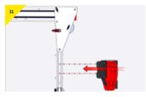
> Present the fall arrest block to the Upright as shown and ensure it is aligned with the holes
