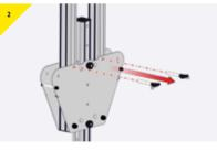
While in this vertical position remove ball lock pin from its stow hole on the Trap Plate.
