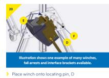
> Rotate winch to align holes, E
