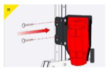
> Insert the retaining pins to secure in place on the Upright
