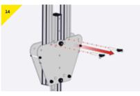
> While in this vertical position remove ball lock pin from its stow hole
