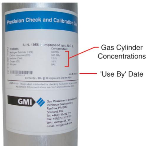
Fig. 2-2 Gas Cylinder Label
