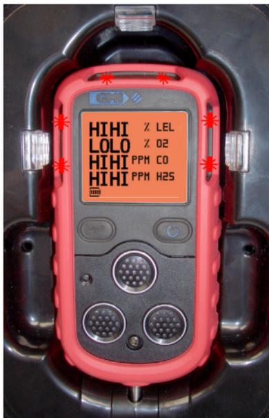
*Fig. 4-11 Instrument in Alarm Condition*
