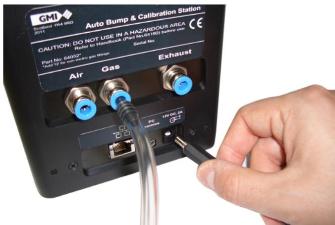
*Fig. 2-8 Connect Power Supply to Station*
