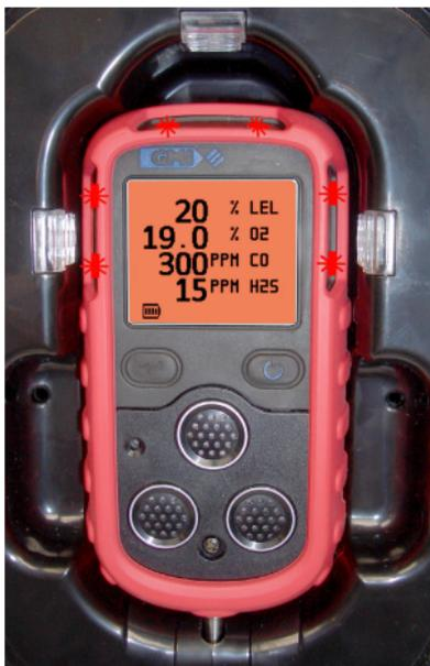
*Fig. 4-10 Instrument in Alarm Condition*
