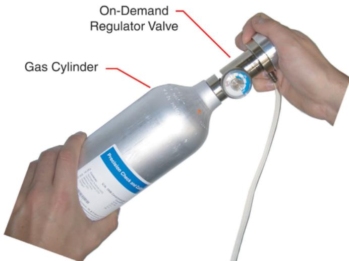
*Fig. 2-4 Attach Regulator Valve to Gas Cylinder*
