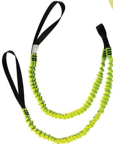
The RTLE4 is an elasticated twin tool lanyard with choke loops for tool attachment. It is suitable for tools up to 5kg in weight.
