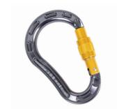
The HMS or belay karabiner has a wide load bearing design allowing for smooth running of your rope. The design also allows the hitch to invert. The karabiner has a screwgate closure.
