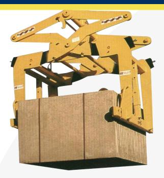
A range of mechanical scissor grabs designed to lift a variety of construction products such as bricks, blocks, kerbs and slabs, both on site and in builder's merchant vards.
