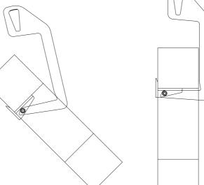
Continue hoisting and traversing the crane until the coil is vertical.take special care when the pivot point is below the cog of the coil as the coil will topple back into the hook, if thin coils are lifted then place the coil down on its edge and move the coil to the rear of the hook for transporting
