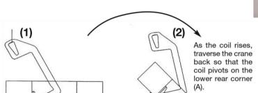
Place the hook into the coil centre as shown above (diagram 1), with the back of the lifting shoe touching the inside of the coil and the lifting sling vertical. Slowly hoist up until the coil rises from the ground.
