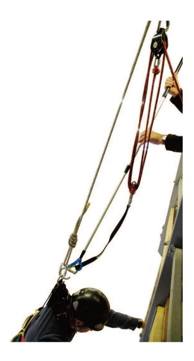
The VRS is designed for the rescue of one person by another individual unassisted. The VRS is for use on a person who has had a fall arrested and is left hanging on a lanyard, webbing or wire rope line. The faller may be raised or lowered to a safe position. When the faller is raised the rescuer has a 4:1 mechanical advantage, which reduces the effort required. The upper pulley wheels lock when the faller is being lowered.
