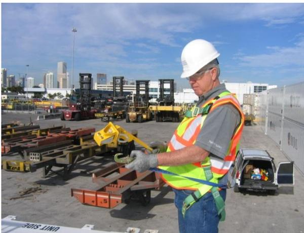
**Connecting the double lock snap of the SRL to the anchor ring of GM120 Top Lock Wand.**
