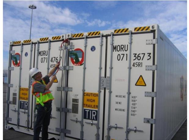
**Inserting head of GM121 End Lock Wand into correct inside edge hole of corner casting.**
