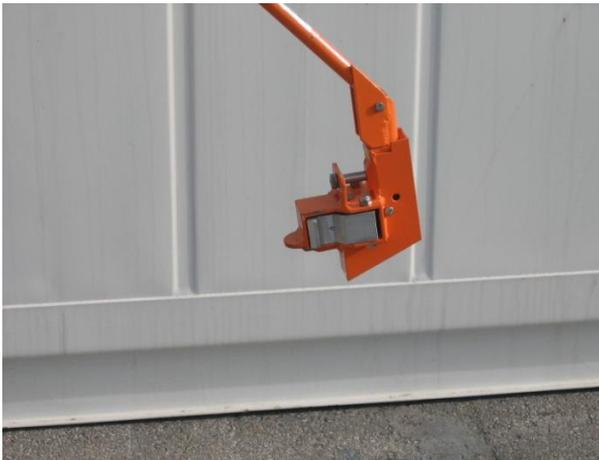
**Head and jaw of the GM184 Top Access End Lock Wand**
