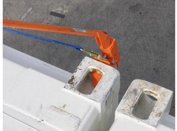
**GM184 Top Access End Lock Wand locked into end hole of corner casting.**
