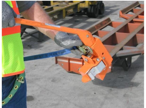
**Connecting a couple lock snap of SRL to anchor point of GM184 Top Access End Lock Wand.**
