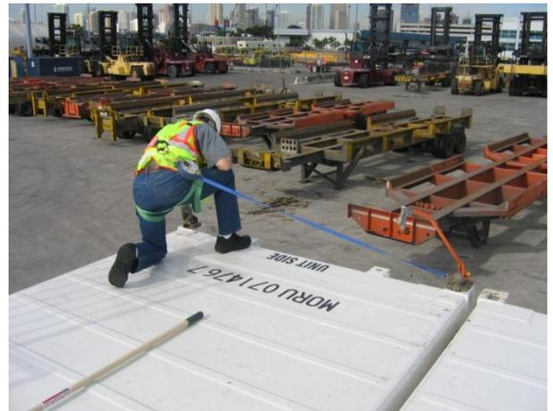
**GM184 Top Access End Lock Wand and twist lock mechanism locked into the same corner casting and worker positioned correctly one container width away.**
