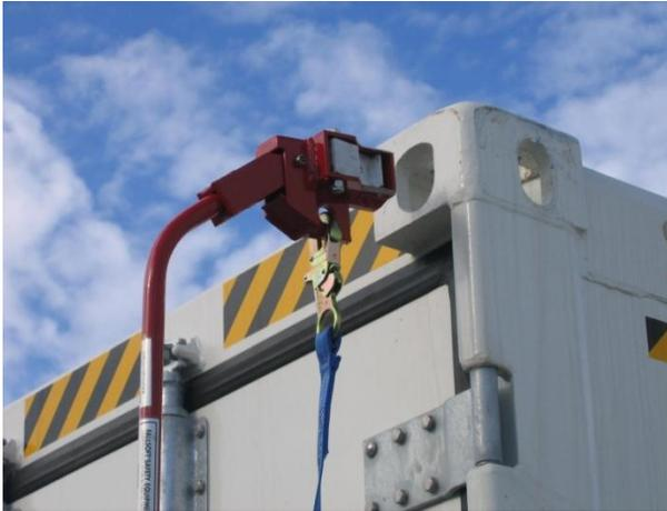
**Inserting head of GM121 End Lock Wand into wrong outside edge hole of corner casting.**
