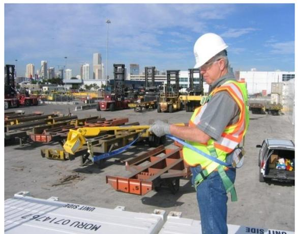
**Extracting sufficient amount of webbing from SRL to allow worker to reach out and insert wand head into corner casting.**
