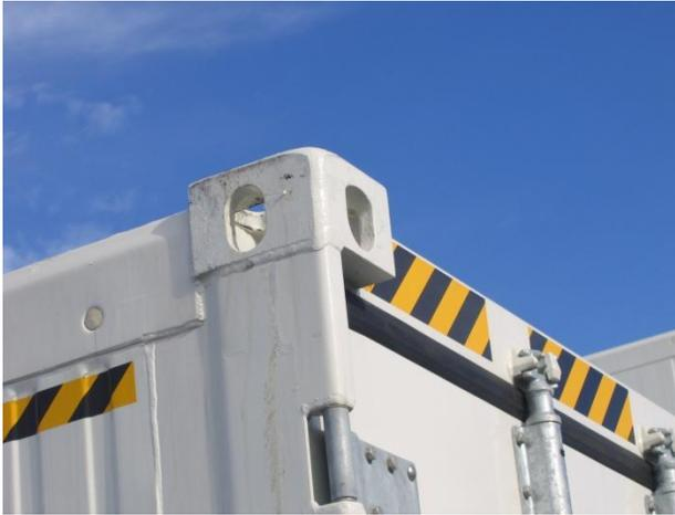
**Corner casting of shipping container showing side hole and end hole.**
