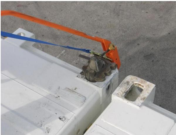
**GM184 Top Access End Lock Wand and container twist lock mechanism locked into same corner casting.**
