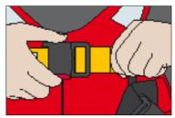
Tighten the top webbing strap by placing one hand on the buckle and pulling the webbing strap with the other hand (illustrated left).
