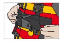
Open the plastic cam buckle and thread the 50mm chest harness through the cam buckle and close ensuring the chest harness is held tight in its grip.
