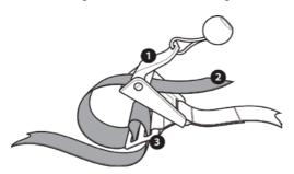
The loose end of the chest harness should be threaded through the metal Tri-glide and cam buckle (illustrated left).
