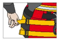
To ensure the PFD is fitted correctly tighten the two webbing straps on each side of the PFD.
