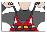
Next, locate the adjustable webbing straps on both shoulders and simultaneously pull each one forward to ensure the correct adjustment and fit. Having followed these steps, the PFD should now fit close to the body.
