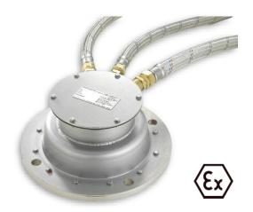
The EM540 Radar employs advanced smart sensor technology packaged with a planar antenna. The radar beam is shaped electronically without the use of additional mechanical parts like lens or horn as seen in traditional radar type level sensors. Versions are available which can be installed either on a still pipe or free space.
