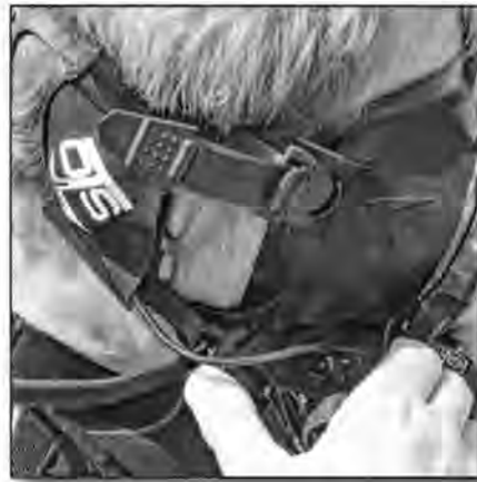
Figure 23: To Remove Mask, Use Thumbs to Grasp Bottom Buckle Tabs and Loosen
