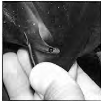
Figure 5: Visor Drain Hole
