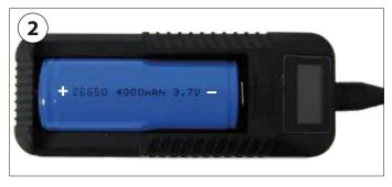
Ensure you insert the battery into the charger the correct way, i.e. with the battery's poles (- and +) touching the corresponding terminals. The correct battery position is labelled on the charger.
