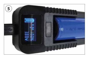
The charger will display the battery's current voltage and overall charging progress. "100%" displayed on the screen denotes that charging is complete.
